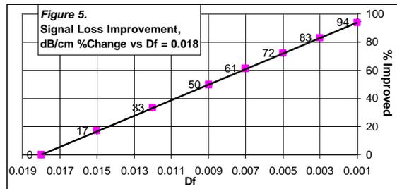
predicts switching from FR4 laminate materials with 0.018 Df to FR408 (Df 0.010) reduces signal loss by 45%.
