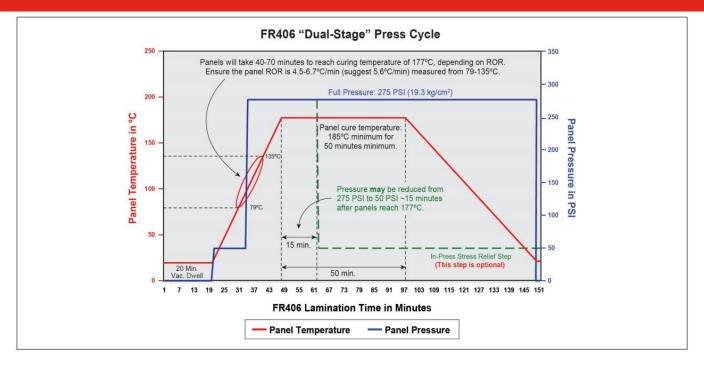
**Please note: This is not a press control program!** The graph represents the preferred pressure/temperature profile panels are subjected to during the lamination program cycle. **Note that the actual high pressure setting and cure duration chosen may differ**
