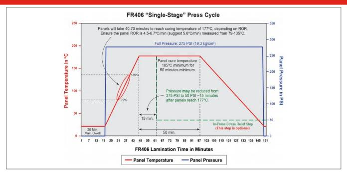
Please note: This is not a press control program! The graph represents the preferred pressure/temperature profile panels are subjected to during the lamination program cycle. Note that the actual high pressure setting and cure duration chosen may differ from the 275 PSI suggested setting shown in this graph. Press pressure and cure duration selected may depend upon board design as well as other factors.
