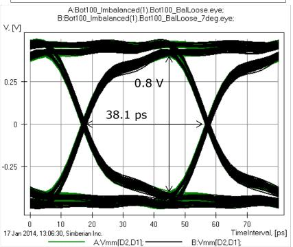
No substantial effect on jitter expected (due to narrow band of the resonance)
