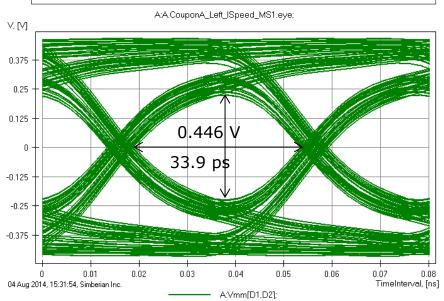
Analysis with Balanced strips produce practically the same eye (no visible difference); Why simulated and measured eyes are slightly different? – see next slide...
