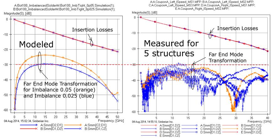
Mode transformation is smaller than expected from the TDR measurements – the imbalance is closer to 0.025
