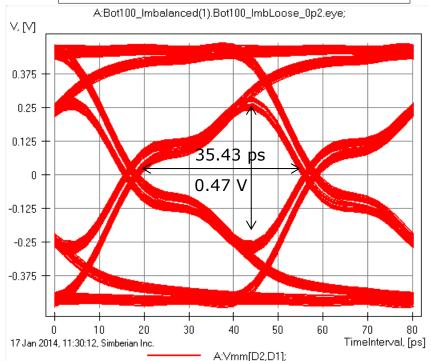
Substantial reduction of eye width (timing jitter) and eye height is expected
