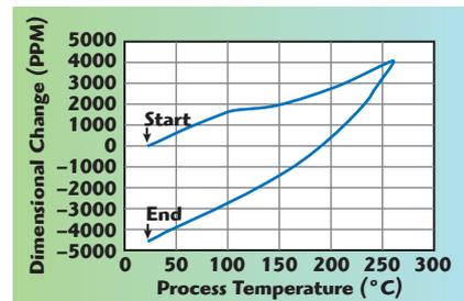
▲ Fig. 6 Y-direction dimensional change versus temperature of microfiber filled PTFE.
