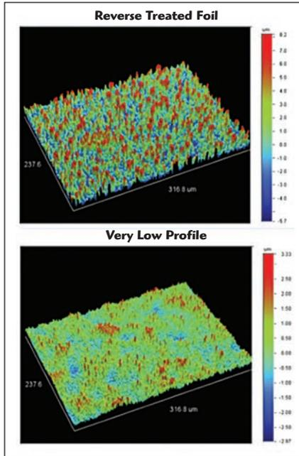
▲ Fig. 1 Comparison of the roughness of reverse treated foil (RTF) and very low profile (VLP) copper. The RTF has a root-mean-square roughness ( $R_{rms}$ ) of  $0.59 \mu\text{m}$ , with maximum height ( $R_z$ ) of  $3.93 \mu\text{m}$ . The VLP is better, with  $R_{rms} = 0.36 \mu\text{m}$  and  $R_z = 2.06 \mu\text{m}$ .
