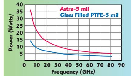
▲ Fig. 11 Maximum power handling of 5 mil, 50 ohm microstrip lines at 85°C for glass filled PTFE and Astra MT300.
