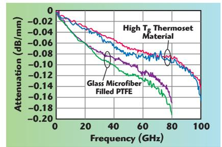
▲ Fig. 10 Attenuation versus frequency of high  $T_g$  thermoset and glass microfiber filled PTFE. Data courtesy of Freescale Semiconductor.
