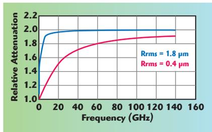
▲ Fig. 3 Relative attenuation as a function of copper surface roughness.
