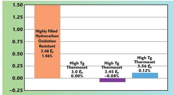
▲ Fig. 8 Change in dielectric constant for various materials, measured at 10 GHz following 1000 hours of aging at 125°C.
