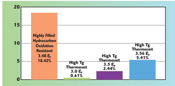
▲ Fig. 9 Change in dielectric loss for various materials, measured at 10 GHz following 1000 hours of aging at 125°C.
