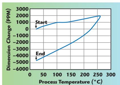
▲ Fig. 5 X-direction dimensional change versus temperature of microfiber filled PTFE.
