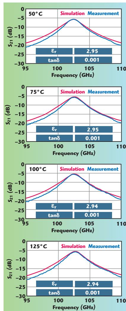
▲ Fig. 7 Simulated and measured RF properties of new thermoset material at various temperatures. Data courtesy of IZM Fraunhofer.
