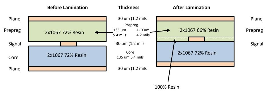
During lamination, the prepreg melts and flows into the areas around copper etched feature. In most SITV's the copper area is very small, so the resin requirement to fill this space is about 90-95% of copper thickness.
