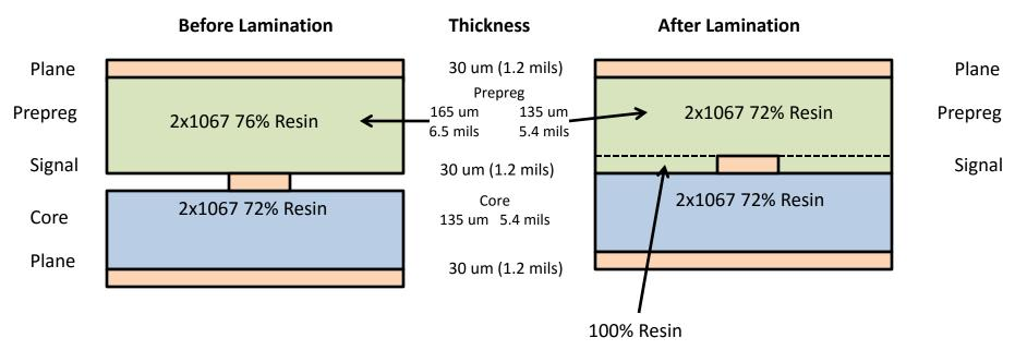
In this approach, the initial prepreg resin content is high, above the target, but after the resin loss into the circuit area, the structure is nearly balanced.
