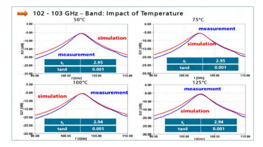
Data generated at IZM Fraunhofer shows stability versus temperature
