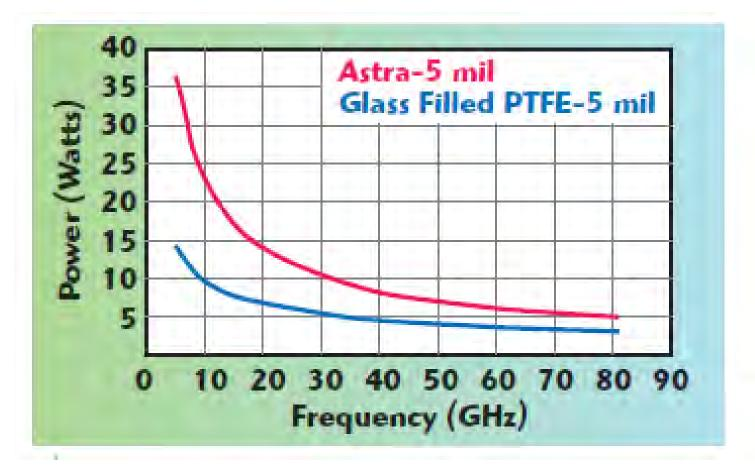
Higher power handling in Astra is enabled by its high thermal conductivity and use of very smooth copper
