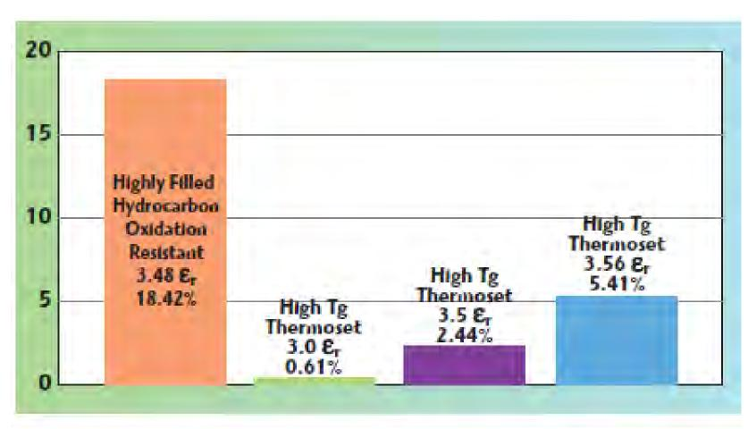
Percent change in dielectric loss after 1000 hours aging at 125°C is shown to be low for high Tg thermosets
