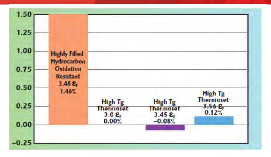
Percent change in dielectric constant after 1000 hours aging at 125°C is shown to be low for high Tg thermosets
