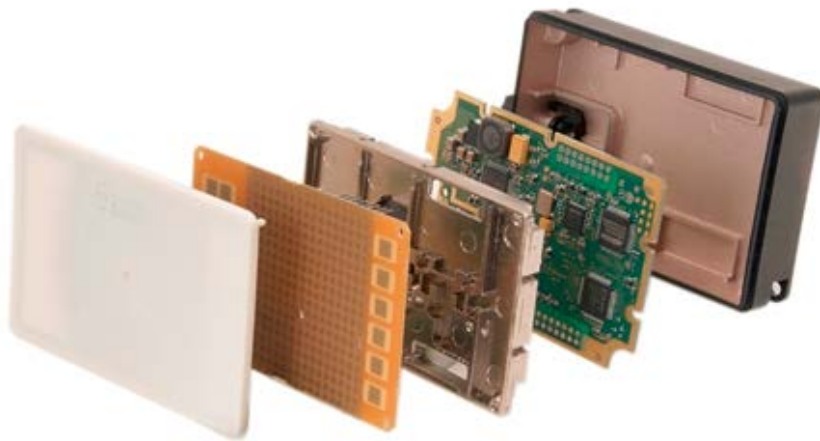
Figure 2: Hybrid constructions allow designers to reduce cost by employing expensive PCB materials for high-performance parts like RF and high-speed digital, while they can use FR-4 for non-critical layers.
